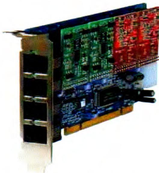
**Figura 15:** Placa TDM400P.
